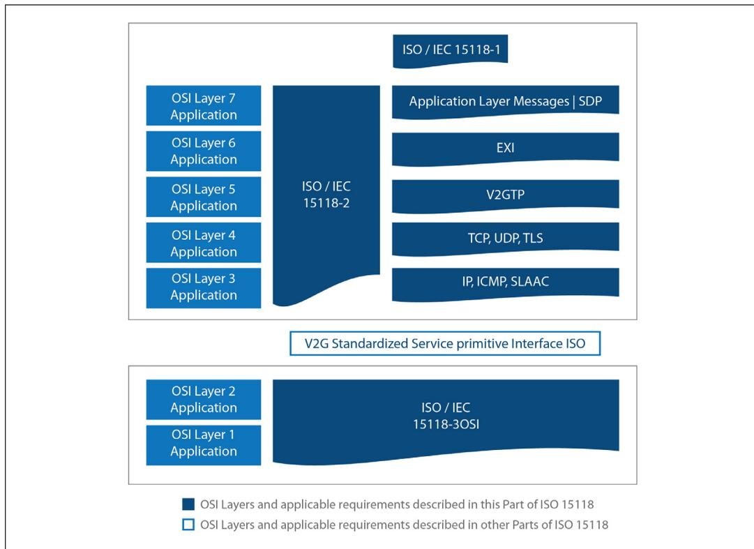
**Figure 2:** Vehicle-to-grid communication (V2G) is based on the ISO/IEC 15118 standard, which can be broken down into three sub-categories.
