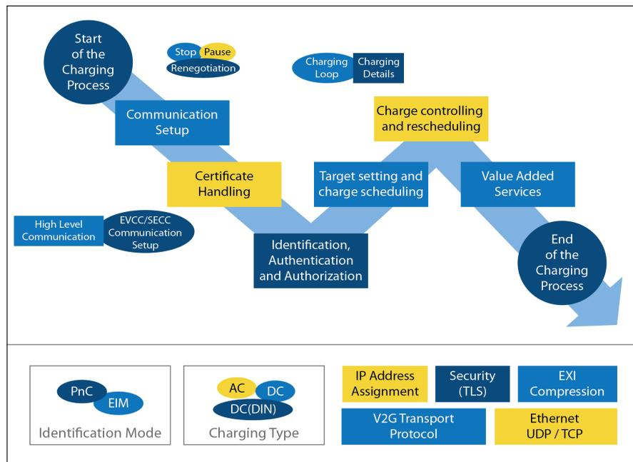
**Figure 3:** Communication between vehicle and charging station.
